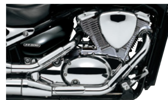
Liquid-cooled, 45-degree V-Twin engine
